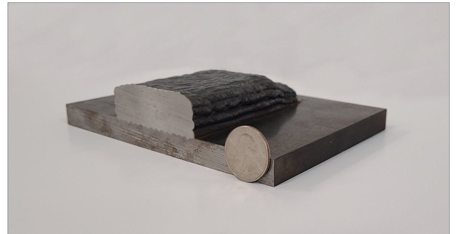
MULTI-LAYER M250 STAINLESS STEEL ALLOY DEPOSITION USING THE CMT, COLD METAL TRANSFER, WELDING PROCESS PERFORMED ON THE WAAM. IT HAS BEEN SECTIONED FOR ANALYSIS.
